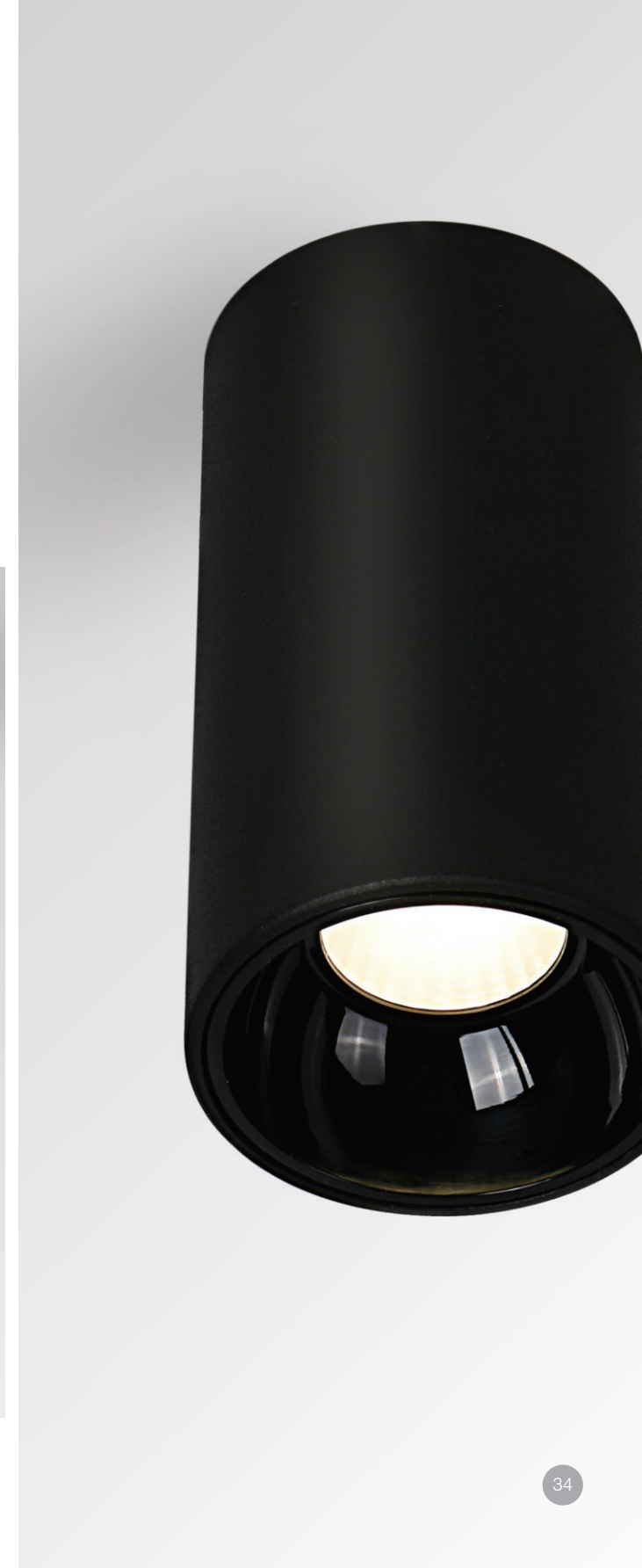
XD2200 30W 2100LM 3000K CRI>80 20° / 45° size Ø116x150mm
