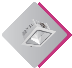
KT6760 10W / 745LM / 50° size 115x115x63mm cutout 105x105mm
